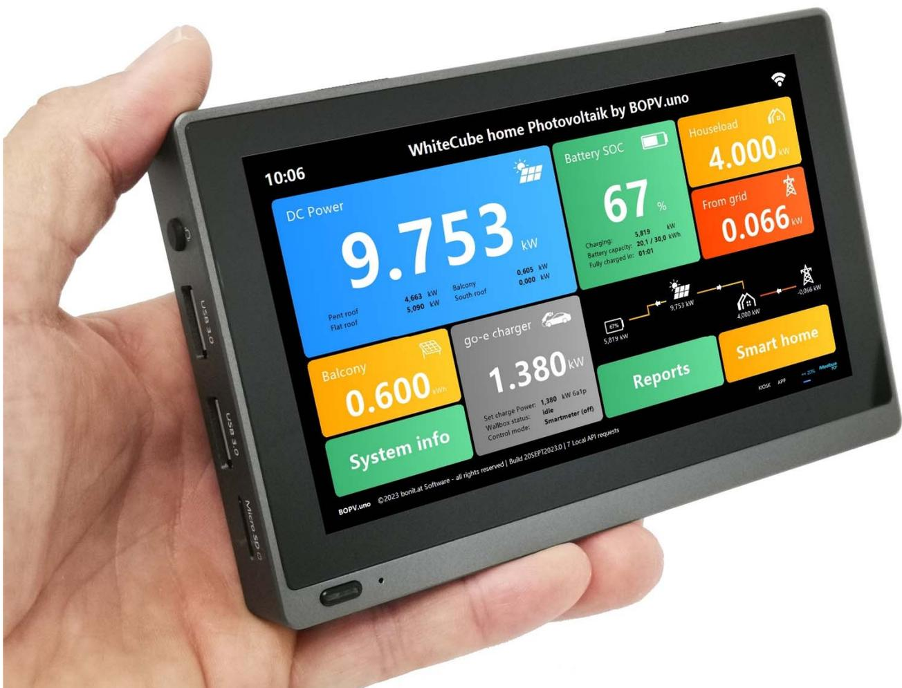
The **BOPV.uno** is designed as a convenient control centre and for the output of real-time data from up to three Huawei, SMA and Fronius inverters and accessories. It retrieves the real-time data from the inverters via Modbus TCP (Huawei/SMA) or V1 API (Fronius). It's easy to configure and use
